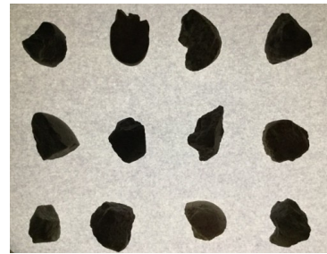
图2 在逆光灯箱条件下拍摄的部分集料 Fig. 2 Pictures of some aggregates taken in backlight light box
